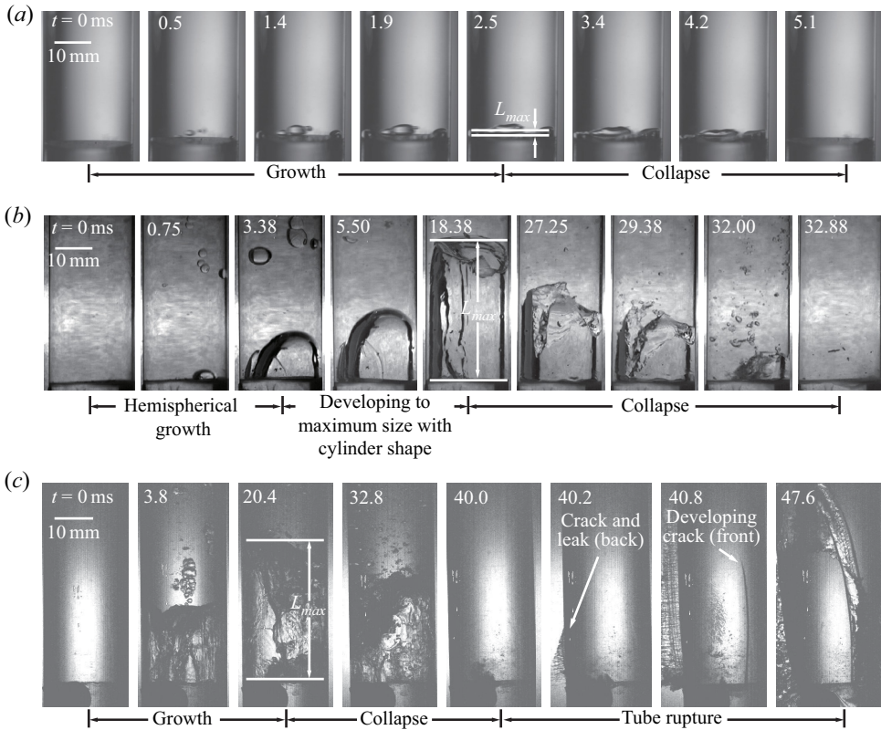
Figure 2. High-speed images of typical cases of cavitation bubble(s) formed at the bottom of the tube. Here, t = 0 ms indicates the moment of tube impacting upon the stopper. (a) Small domed cavitation bubbles. (b) Large cylindrical cavitation bubble. (c) Tube burst caused by the collapse of a large cavitation bubble. Here, d = 18, 16, 18 mm, l = 200, 530, 640 mm, u_0 = 1.91, 3.40, 3.08 m s -1 and a = 843.00, 1857.00, 8050.00 m s -2 , for case (a), (b) and (c), respectively.
