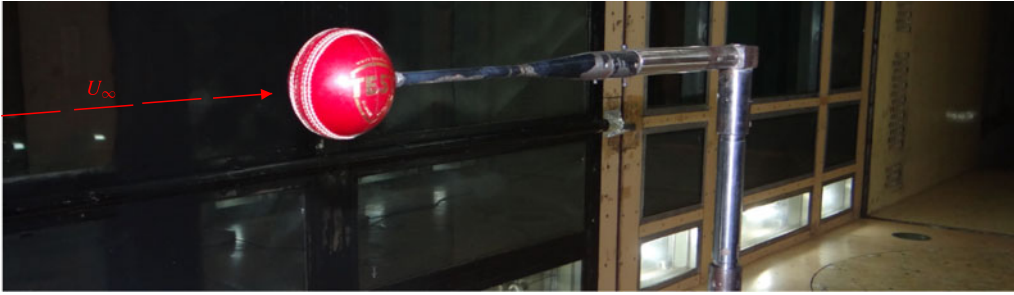
FIGURE 3. (Colour online) An SG Test cricket ball shown mounted on the experimental set-up in the wind-tunnel test section.
