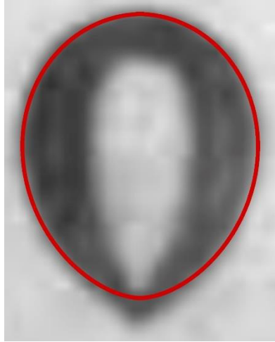
Figure 6. For a bubble of \tilde{R}_b = 2.7 mm in the 1.5 % polyox solution, comparison between the steady-state experimental shape by LLJ with our prediction indicated by the continuous red line.
