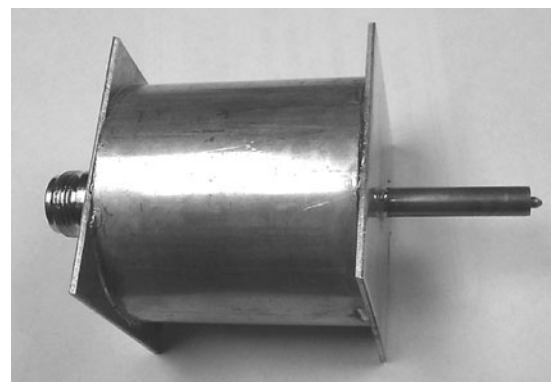
Fig. 10. Completed second test case cavity.
