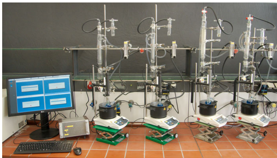
Fig. 3. Four simultaneously operated and jointly controlled WDAs. The control electronics can be seen on the left.
