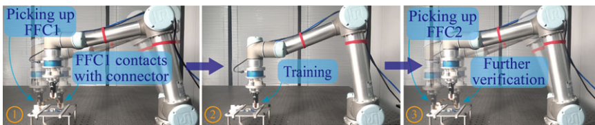
Figure 8. The procedure of the FFC assembly experiment.
