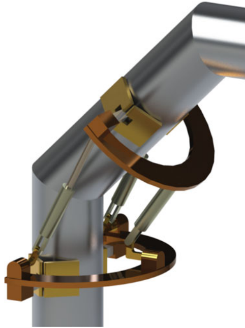
Fig. 12. Illustration of the Wide-Open robot in a pole-climbing application. The robot is frontally open where it can easily embrace tubular objects. It can travel along tubular structures with bends, branches, and step changes in cross section. It is also able to perform manipulation, repair, and maintenance tasks after reaching the target point on the structure.
