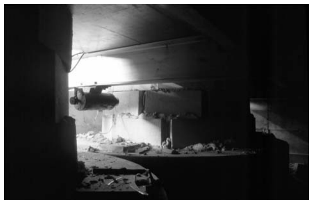
Figure 3. Mechanical oscillator mounted under floor plate.
