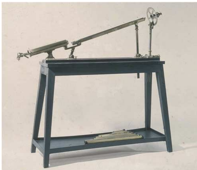
Figure 2. (Colour online) Picture of a polarimeter kept at the Pasteur museum. A polarimeter is an instrument allowing one to observe and measure the action of a compound on polarized light.
