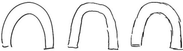
Fig. 3. Examples of line work that are: clean, with tremor, and with hash marks (left to right).
