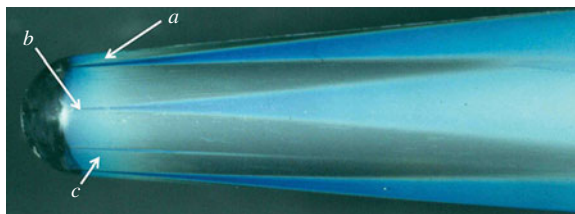
FIGURE 1. Thermochromic liquid crystal image of turbulent wedges on a blunt cone, from Zanchetta (1996).
