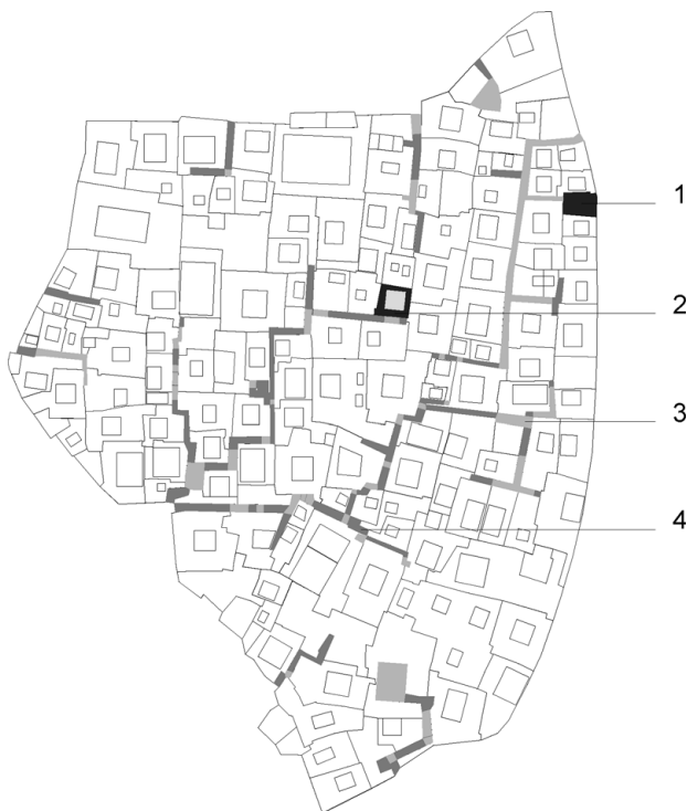
Fig. 2. The plan of Zaouiat Lakhdar. (1) The lots bordering the outer streets are mainly used for shops and public facilities. (2) The inner lots are accessed by (3) narrow, zigzagged, dead-end streets, called derbs , which are occupied by patio houses. The derbs are partially covered by (4) sabbats .
