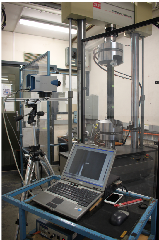
Figure 26. Specimen installed in the servo-hydraulic test machine and the infra-red camera.
