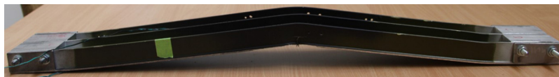
Figure 18. Simulated corrosion Specimen 2 after testing showing the effect of the localised buckling.
