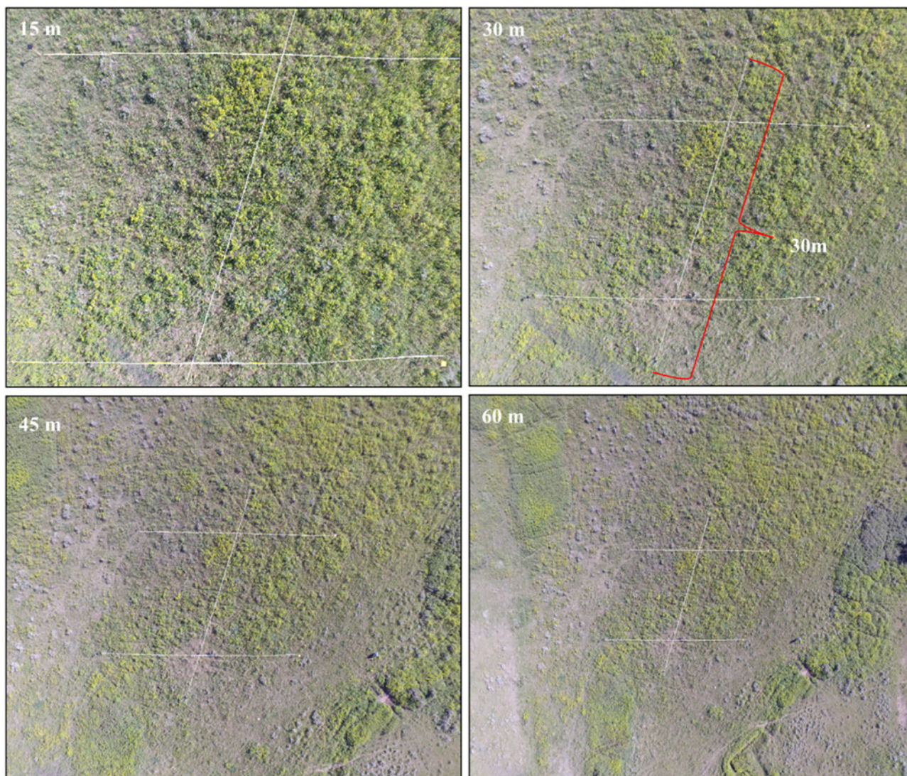
Figure 3. Unmanned aerial vehicle red-green-blue images acquired between 9:12 and 9:15 AM at four different flight heights (ranging from 15 to 60 m) for site 1. In each image, the white lines are the measuring tapes placed along the ground-vegetation sampling transects.
