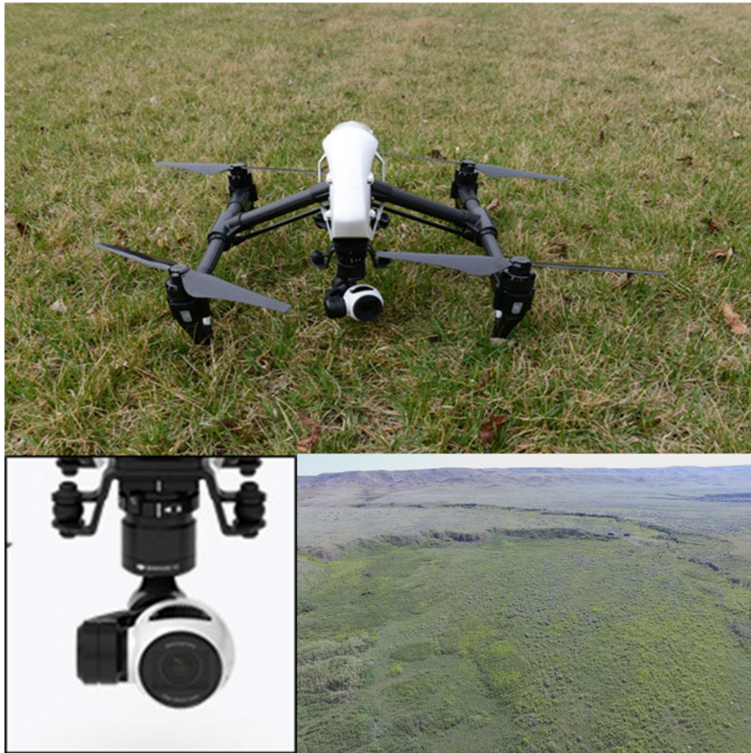
Figure 2. The unmanned aerial vehicle system (top), camera (bottom left) and true color image of the site (bottom right).
