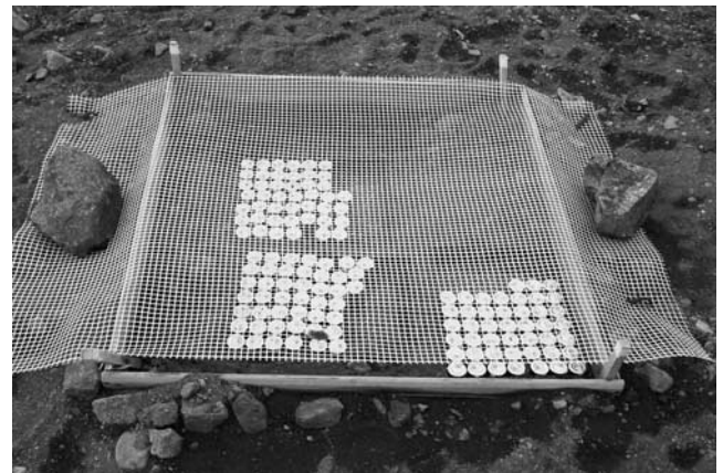
Fig. 2. View of the experimental system exposed to environmental conditions at Jubany Station. Three metal trays containing 21 microcosms each were located in the field, protected by a wood frame and covered with a plastic net.
