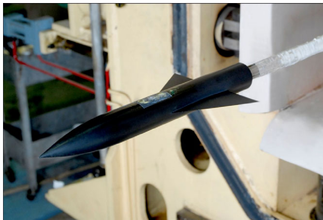
Figure 2. Photograph of the AGARD-B model mounted in the tunnel test section.
