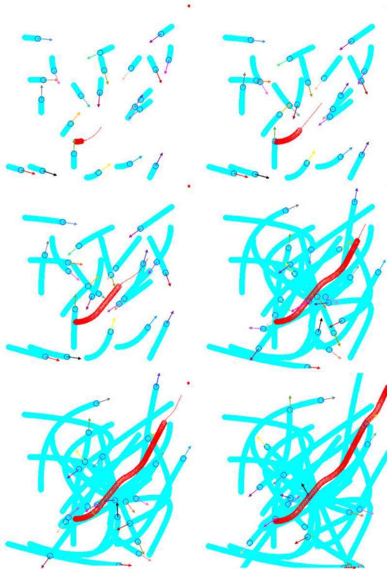
Fig. 12. PASSPMP-PSO at work in a crowded environment: sequences of \mathcal{A} 's displacement at different instants of the process. The red mark left behind the robot is the executed trajectory. The trajectory ahead the robot is the planned trajectory (to be executed). The marks in cyan behind the objects represent their displacement and the arrows depict the directions of their trajectories, where each object is assigned an arrow colour (for a better visualization of their position with time).
