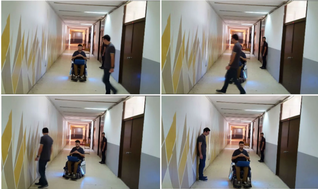
Fig. 21. PASSPMP-PSO at work in the presence of a moving object, sequential snapshots of wheelchair motion (from top left to bottom right). When the pedestrian is detected, an arbitrary collision-free braking trajectory is executed (the first two snapshots). In the third snapshot, the wheelchair is at rest. In the last snapshot, the wheelchair has pursued its trajectory as the passage is free.
