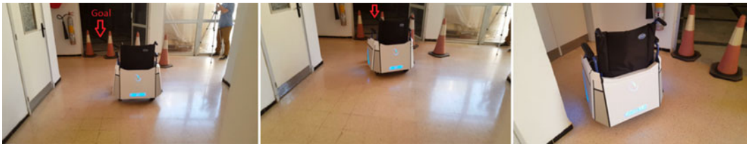
Fig. 22. PASSPMP-PSO's behaviour in a dead-end situation. A collision-free braking trajectory is executed to guarantee p-safety. In the last snapshot (on the right), the wheelchair is at rest (there is no issue, even at rest).
