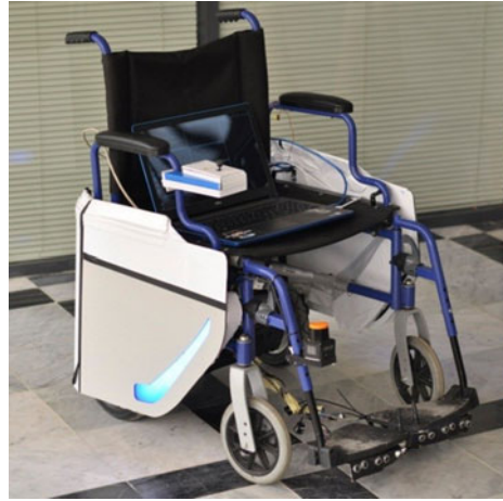
Fig. 18. Experimental platform; a robotic wheelchair.
