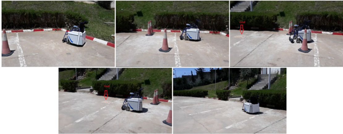
Fig. 19. PASSPMP-PSO at work in an outdoor environment; sequential snapshots (from top left to bottom right) of wheelchair motion towards a goal while passing through a narrow passage (the red arrow designates the goal).
