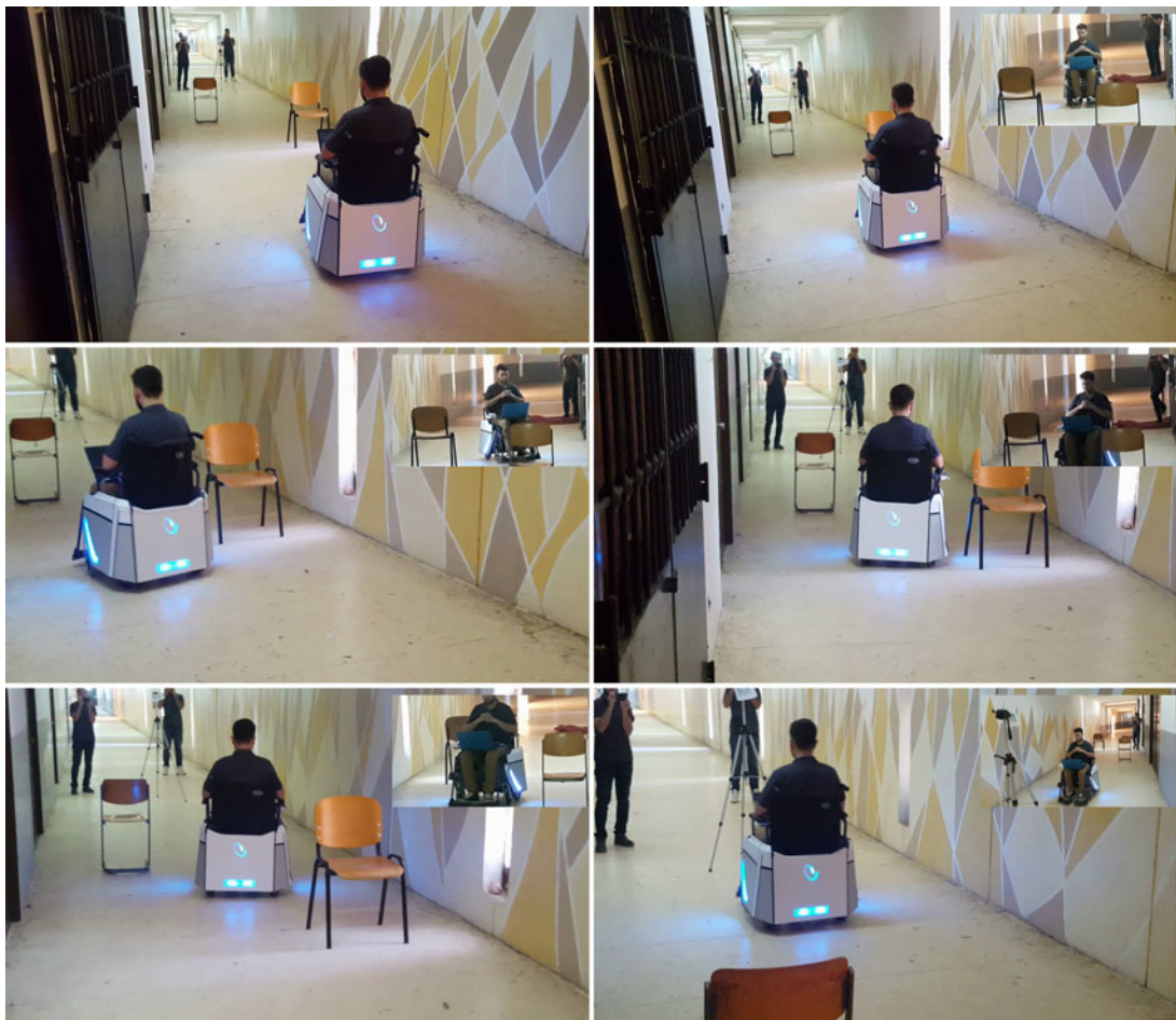
Fig. 20. PASSPMP-PSO at work in an indoor environment. Sequential snapshots of wheelchair motion (from top left to bottom right); it evolves in a corridor and reaches its goal while avoiding static objects. The goal is just before the tripods.
