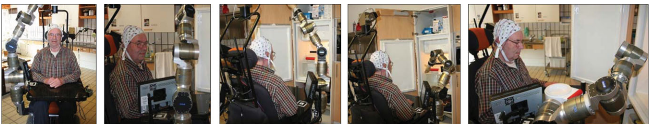
Fig. 11. (Colour online) Sequences of robotic operations within the “prepare and serve a meal” support scenario during testing at the NRZ rehabilitation center.
