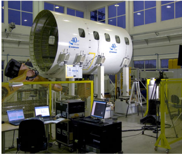
Figure 1. Partial view of the ASAA fuselage assembly cell.
