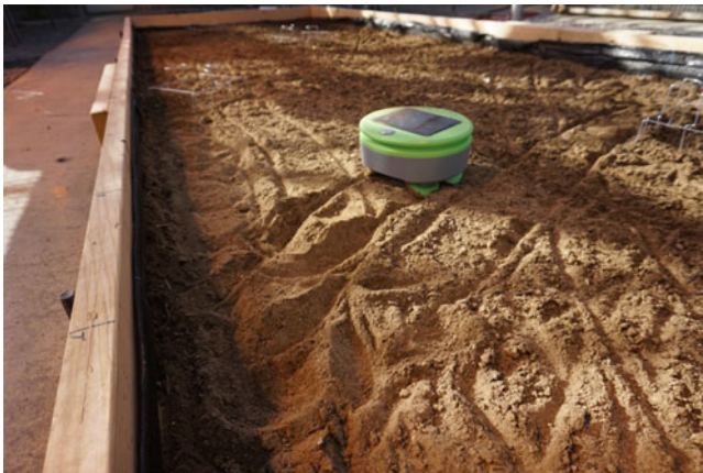
Figure 2. Soil disturbance caused by grousers.
