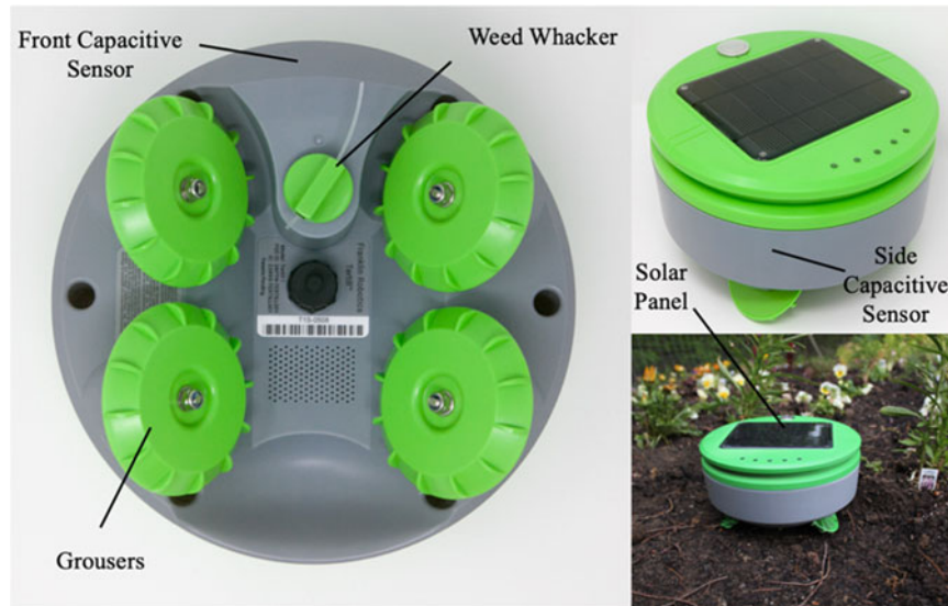
Figure 1. Underside of the Tertill™, showing four wheels or “grousers,” weed-whacking mechanism, capacitive sensors, and solar panel.
