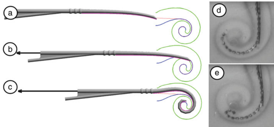
Fig. 3. Advance Off Stylet insertion technique. (a) The PEA is inserted until the distal end reaches the basal turn. (b) Stylet retraction is coordinated with continued insertion into the scala tympani. (c) At full insertion depth the stylet is completely. (d) Normal insertions result in the PEA electrodes being in close contact with the modiolus. (e) Tip-folding results in the distal tip of the PEA bending over itself inside the cochlea.
