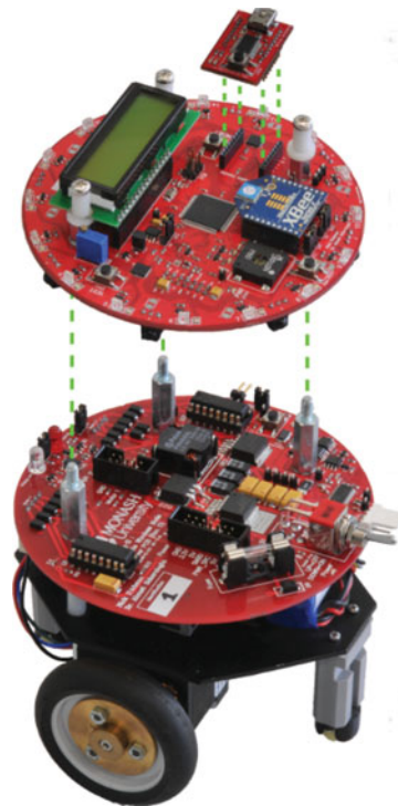
Fig. 6. Experimental robot eBug. It has a diameter of 120 mm and is equipped with two stepper motors driving two wheels independently. Further details about its hardware and firmware can be found in. 13
