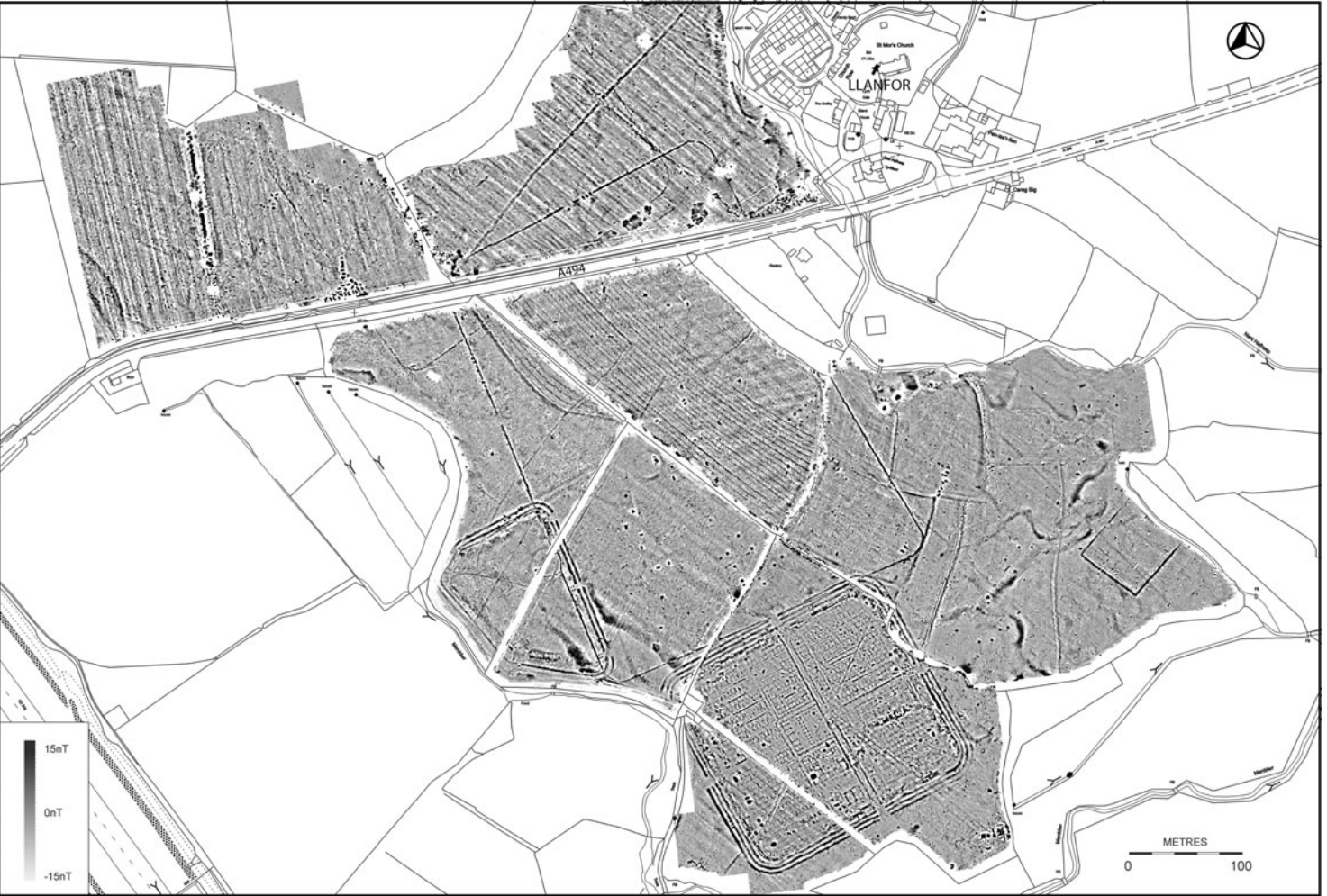
FIG. 3. Gradiometer survey of the Llanfor military complex. (Background map © Crown copyright Ordnance Survey. All rights reserved)
