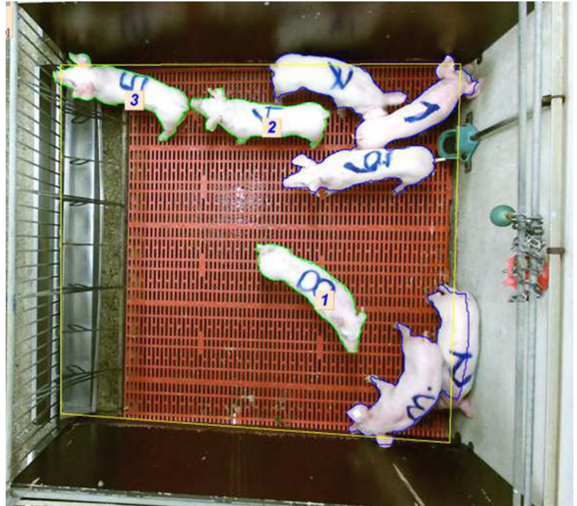
Fig. 1. Image of a piglet group generated by the program for image analysis. Animals identified as individuals have a green line drawn around them and are numbered 1–3. Picture: CLK GmbH (Altenberge, Germany).
