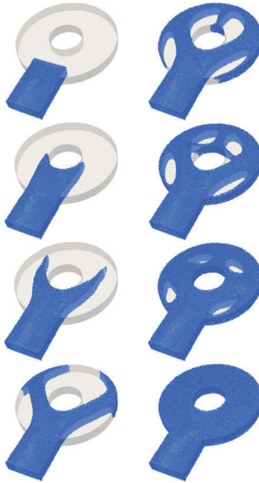
FIGURE 9. 3D Mould filling patterns for Re = 210 at different time steps predicted by FPM.
