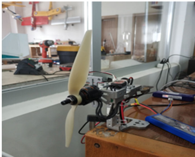
Figure 2. Test stand prepared to obtain dataset.
