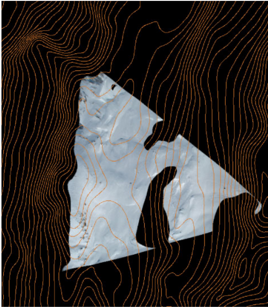
Fig. 6. Georeferenced map of reflectance values from digital photographs taken from Pic du Lac Blanc (at the lower right of the image) in the direction of Col du Lac Blanc (at the lower centre left of the image). This map was acquired after the correction for terrain parameters, atmospheric transmittances and the ratio of direct to diffuse radiation produced in Figure 7.
