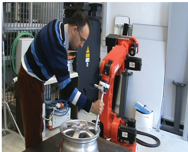
Fig. 7. (Colour online) The operator interacting with the robot during a walk-through programming operation.
