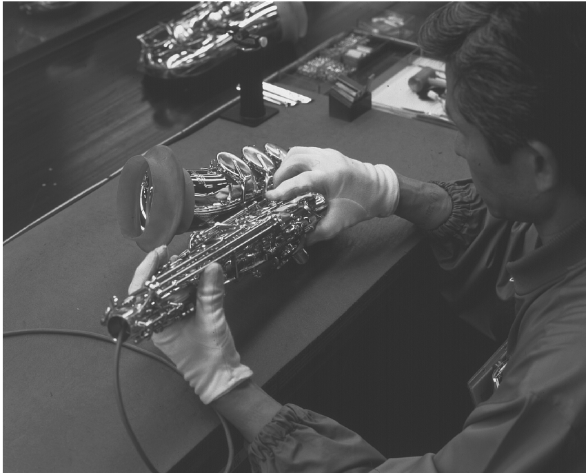
Fig. 2.9 Testing for the integrity of pad seating on a Yamaha saxophone
