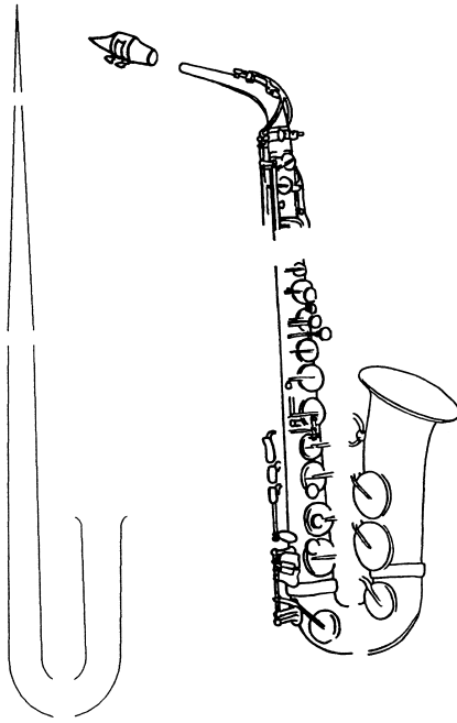
Fig. 2.3 Viewing a design sketch to incorporate four cones and their relationship with the complete saxophone
