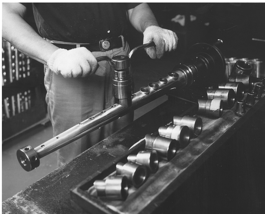
Fig. 2.8 Toneholes being raised from a saxophone tube at the Yanagisawa factory in Japan
