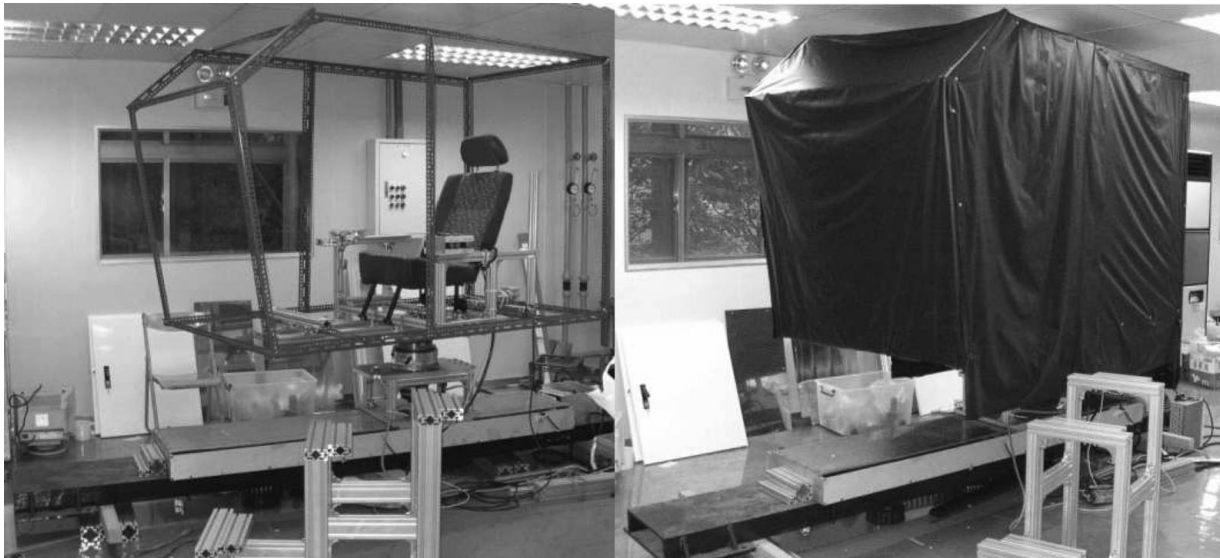
Fig. 5. Photo of the 2-axis motion simulator with VR environment.
