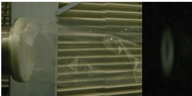
Fig. 12. (Color online) Photographs of window RF breakdown in the atmosphere with a clear plastic bag filled with SF 6 .
