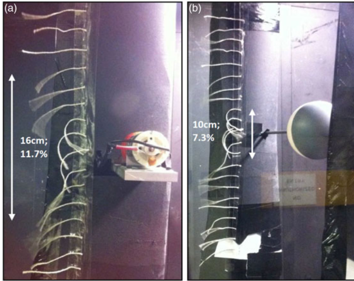
Figure 9. Wake regions produced by (a) active and dummy motor and (b) shaft.
