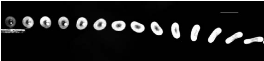
FIGURE 15. Toroidal glycerol marble leaving its substrate and falling freely in air. We observe a spontaneous (and irreversible) transformation towards a two-lobed shape. 4 ms separates each image, the drop has an initial radius R_0 = 2.1 mm and the bar represents 1 cm.
