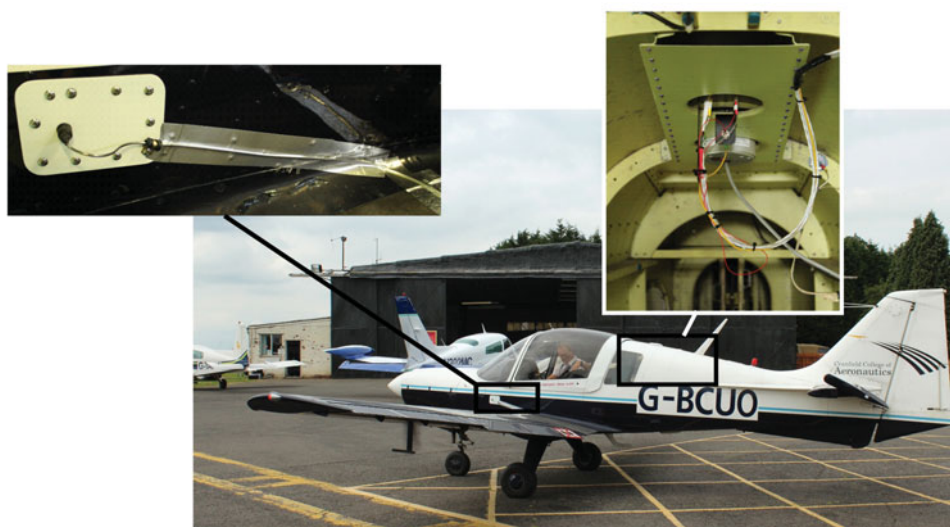
Figure 6. (Colour online) Image of the Bulldog showing the routing of the fibre optic systems through the fuselage.
