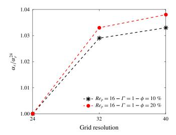
FIGURE 2. (Colour online) The effective thermal diffusivities, normalized by the value of  $\alpha_r$  for 24 grid points per particle diameter ( $\alpha_r^{24}$ ), versus grid resolution per particle diameter.
