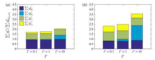
FIGURE 14. (Colour online) Wall-normal integral of the different terms defining the average heat flux across the channel, normalized by the total heat flux in single-phase flow for: (a)  $\phi = 10\%$  and (b)  $\phi = 30\%$ .
