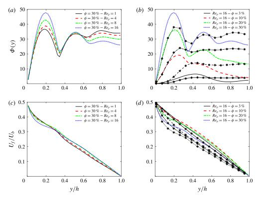
FIGURE 8. (Colour online) Local volume fraction  $\Phi(y)$  and the mean streamwise velocity of the fluid versus the normalized distance to the wall y/h for (a,c) the different particle Reynolds number under investigation at  $\phi = 30\%$  and (b,d) different volume fractions at  $Re_p = 16$ . The results for non-rotating particles are indicated with the same line style as their rotating counterparts, using asterisks in (b) and (d).
