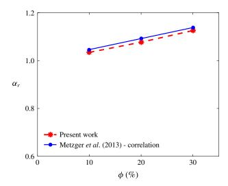
FIGURE 4. (Colour online) Effective thermal diffusivity, normalized by the thermal diffusivity of the single-phase flow,  $\alpha_r$ , for the different volume fractions under investigation. The parameters for these simulations are set to Pr = 20, 2h/D = 6,  $Re_p = 0.5$  and  $Pe = Re_p Pr = 10$ .
