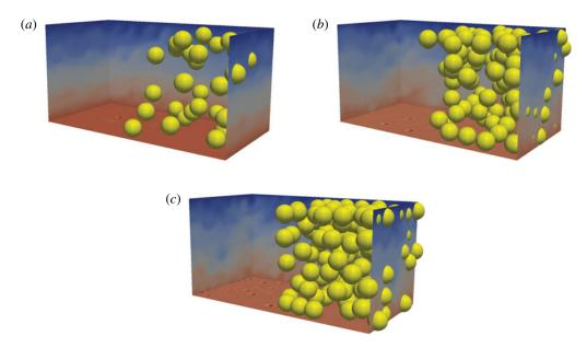
FIGURE 5. (Colour online) Snapshots of the temperature in the suspension flow for the volume fractions  $\phi = 10$ , 20 and 30% at  $Re_p = 16$ .
