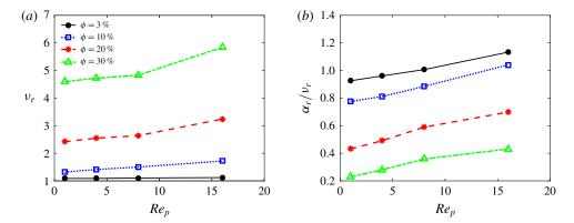
FIGURE 7. (Colour online) (a) Effective viscosity of the suspension normalized by the viscosity of the fluid and (b) the ratio between the increase of the heat transfer  $\alpha_r$  and the increase of the suspension effective viscosity  $\nu_r$ .
