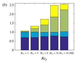
FIGURE 11. (Colour online) Wall-normal integral of the heat fluxes transferred by different mechanisms, normalized by total heat flux in single-phase flow for: (a)  $\phi = 10\%$  and (b)  $\phi = 30\%$ .
