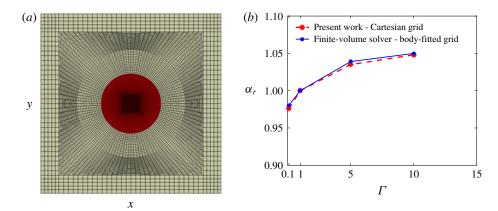
FIGURE 3. (Colour online) (a) A two-dimensional section of the boundary-fitted orthogonal grid used in the finite volume solver. (b) Effective thermal diffusivity  $\alpha_e$  normalized by the thermal diffusivity of the fluid  $(\alpha_r \equiv \alpha_e/\alpha_f)$  for different thermal diffusivity ratios  $\Gamma$  between the particle and the fluid.
