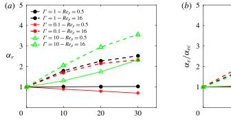
FIGURE 12. (Colour online) (a) The effective thermal diffusivity of the suspension, normalized with that of the single-phase flow,  $\alpha_r$ , versus the particle volume fraction  $\phi$  and (b) the same data normalized with the effective thermal conductivity of a composite ( $\alpha_{ec}$ ) with the same volume fraction, estimated according to the Lewis–Nielsen model (Nielsen 1974).
