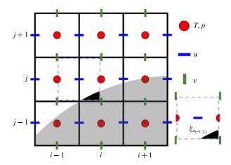
FIGURE 1. (Colour online) The staggered Eulerian grid and the phase indicator  $\xi$  around the velocity point  $u_{i-1/2,i}$ .
