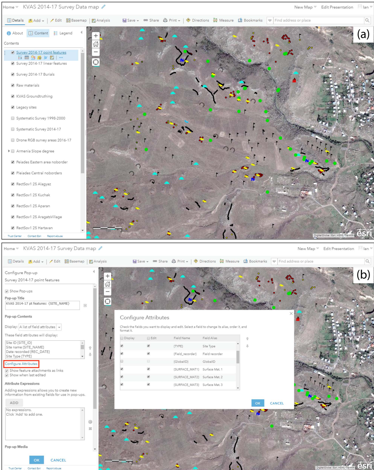
FIGURE 5. Project web map viewer in ArcGIS Online: (a) web map with feature service and image service layers; (b) configuring pop-ups to determine how editable layers and menus will appear to end users in ArcGIS Collector. (In our case, the web map is populated with sites from the survey, but a new web map would, of course, be empty.)
