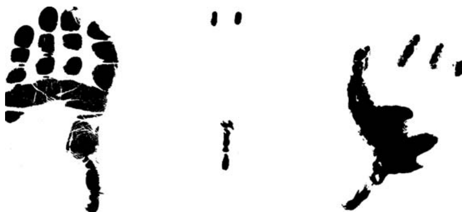
Fig. 4a–c. Contact areas between a bottle and a natural hand (left), an Otto Bock System Electrohand (middle) and the multifunctional prosthetic hand (right).
