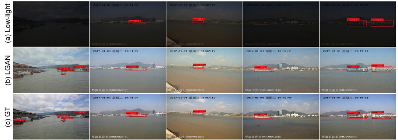
Figure 9. Vessel detection experiments on synthetic low-visibility maritime images (a). Vessel targets are not easily detected in the synthetic low-illumination images. After enhancement by LGAN (b), the target detection results are very close to ground truth (GT) (c).
