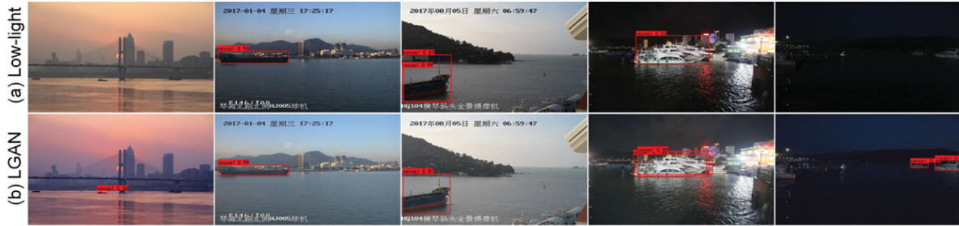
Figure 10. Vessel detection experiments on real maritime images (a). Some vessels are not detected on real low-visibility images and there is a problem of repeated detection. In contrast, using LGAN to pre-process low-visibility images can significantly improve the robustness and accuracy of vessel detection (b).
