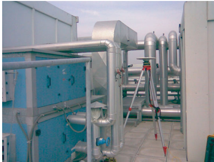
Figure 1. Point A in a potential multipath environment.
