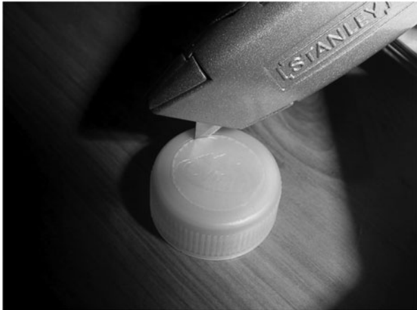
FIG. 2 Making the perforations.
