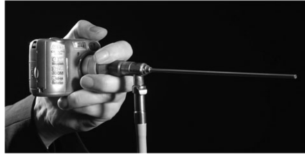
FIG. 4 Endoscope mounted on camera with adaptor.
