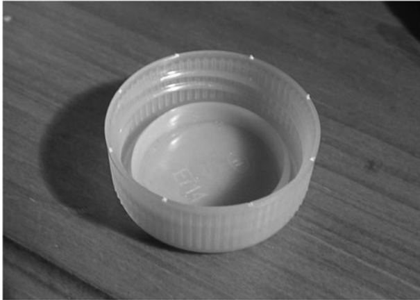
FIG. 1 Evian plastic mineral water bottle top, showing inner ring.
