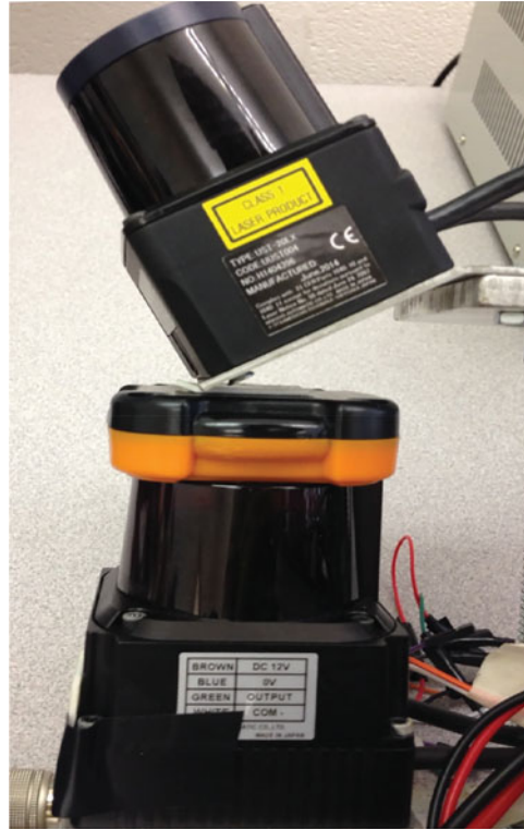
Figure 11. Hokuyo lasers and IMU (LADAR1 on the bottom and LADAR2 on the top).
