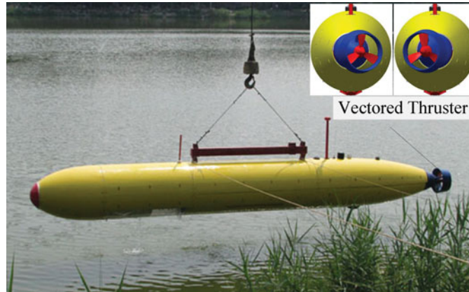
Fig. 3. Tianjin University's AUV equipped with a vectored thruster.
