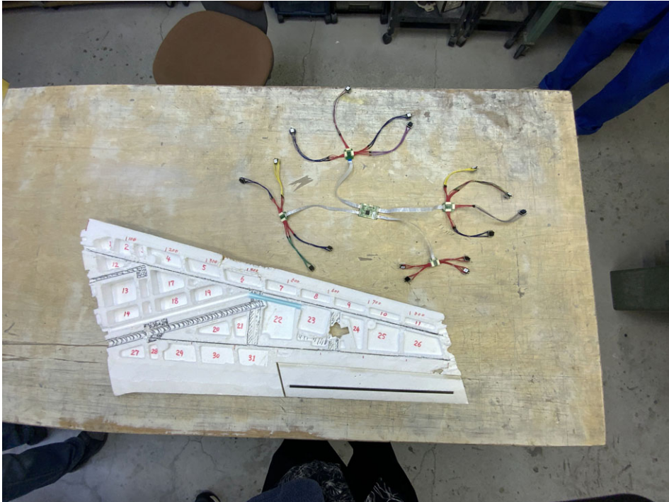
Figure 3. Tearing open the wing to examine its internal structure and assess potential space for electronic component wiring. Due to its weaker structural strength, the half-cut wing in the photo was not used in the experiment.
