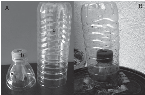
Fig. 1. The emergence trap. (A) Components of the trap: (a) 7-cm cut section; (b) bottle cap with 1-cm hole; (c) 15-cm cut section. (B) Completed trap.
