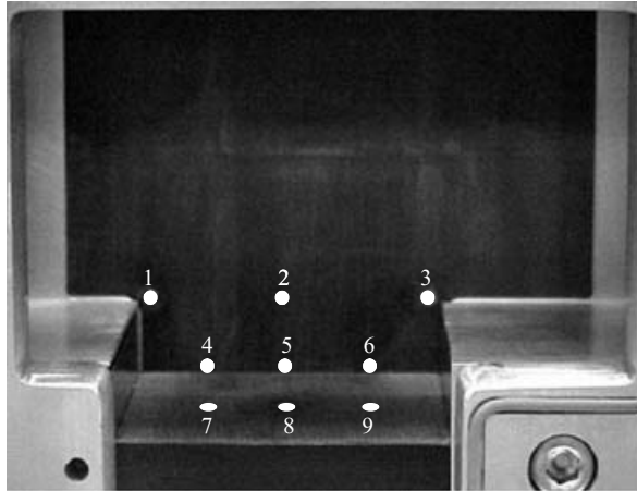
FIGURE 2. Position of the Kulite pressure transducers 1–6 (on the sidewall) and of transducers 7–9 in the cavity floor.
