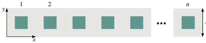
FIGURE 4. (Colour online) Solution domain for the DNS consisting of an array of n inline square unit cells of length \ell .
