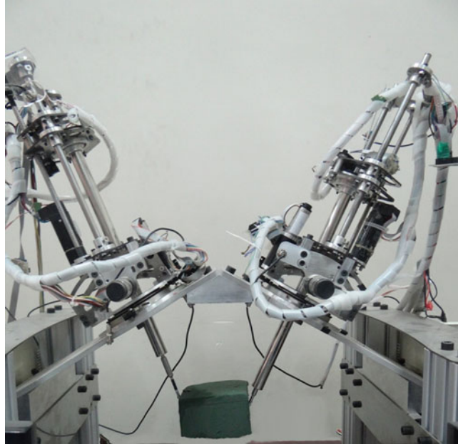
Fig. 13. 4-DOF RRPR surgical manipulator.
