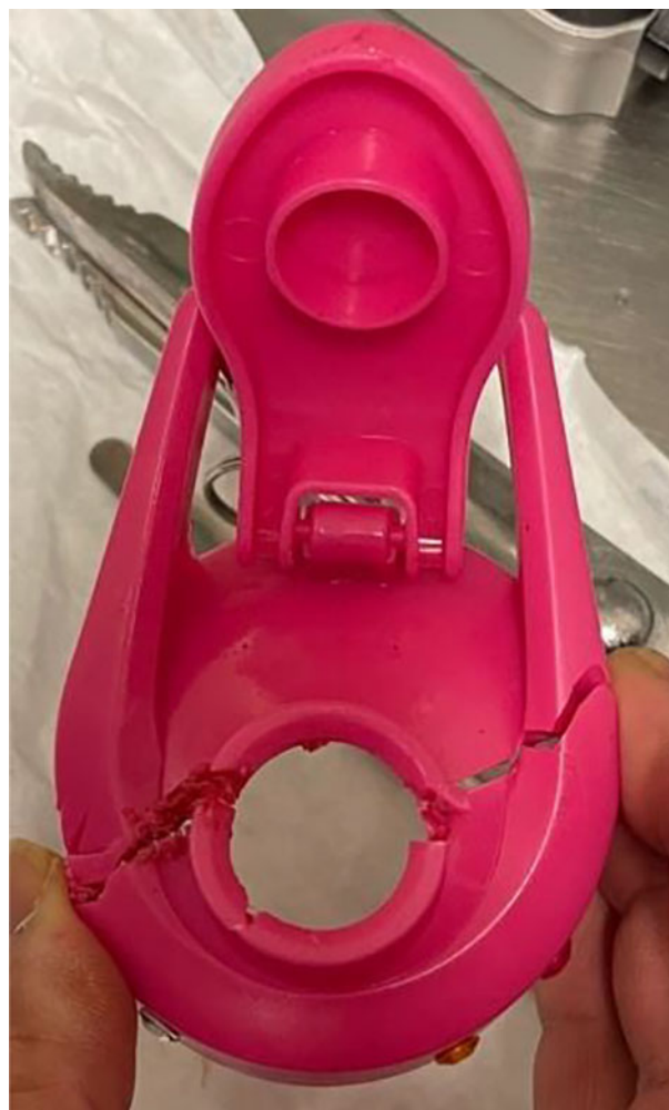
Fig. 2. Oblique incision through the bottle lid (left side).
