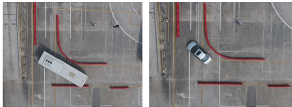
The Guangzhou Comprehensive Street Design Handbook tested turns of 4m, 5m, 8m, 10m and 12m radius with cars, 9-metre buses and 12-metre buses (Image: Guangzhou City Planning Design and Research Institute)
