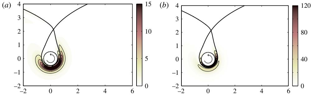
FIGURE 10. (Colour online) Structural sensitivity  $\mathbf{S}_b$  for  $Re = 100$ ,  $\alpha = 5$ : (a)  $\kappa = 0$ ; (b)  $\kappa = 1$ . The black curve shows the streamlines passing through the stagnation point. The contour spacing is (a) 3, (b) 24.
