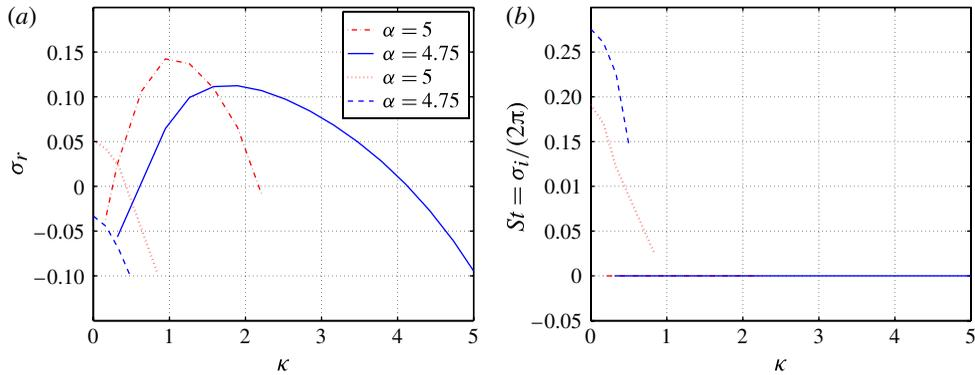
FIGURE 1. (Colour online) Growth rate  $\sigma_r$  (a) and Strouhal number  $St = \sigma_i / (2\pi)$  (b) for  $Re = 100$  as a function of the rotation rate  $\alpha$  and spanwise wavenumber  $\kappa$ . The stationary modes are indicated by the solid lines while the unsteady modes by the dashed lines.
