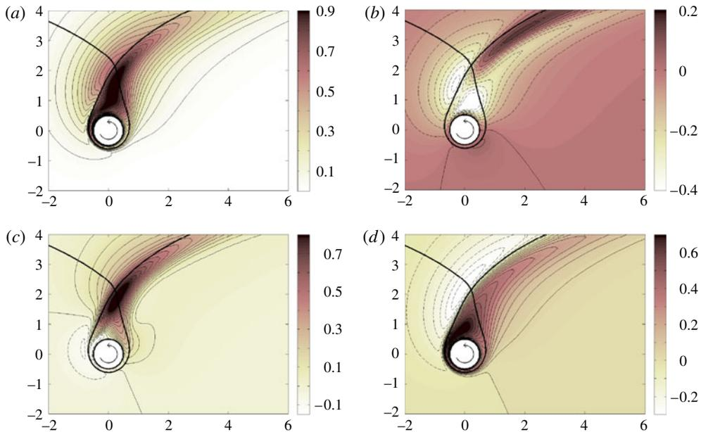
FIGURE 7. (Colour online) Spatial structure of the perturbation velocity at  $Re = 100$ ,  $\alpha = 5$  and  $\kappa = 1$ : (a) modulus; (b) horizontal component  $u$ ; (c) vertical component  $v$ ; (d) spanwise component  $w$ . The mode has been normalized such that the maximum of the modulus is 1. The contour spacing is 0.05 and continuous lines are positive values while dashed lines are negative values.
