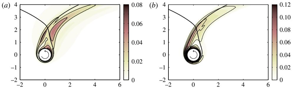
FIGURE 6. (Colour online) Modulus of the perturbation vorticity  $|\omega(x, y)|$  at  $Re = 100$  and  $\alpha = 5$ ;  $\kappa = 0$  (a) and  $\kappa = 1$  (b). The black curve shows the streamlines passing through the stagnation point. The contour spacing is 0.02.
