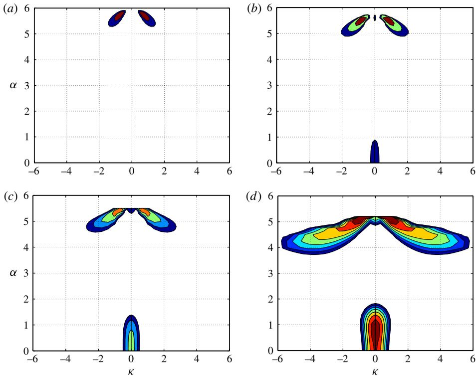
FIGURE 2. (Colour online) Growth rate  $\sigma_r \geq 0$  in the plane  $(\alpha, \kappa)$ : (a)  $Re = 40$ ; (b)  $Re = 50$ ; (c)  $Re = 60$ ; and (d)  $Re = 100$ . The contour spacing is 0.02 in all figures.
